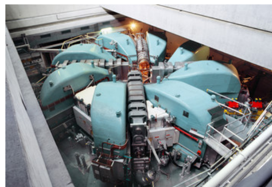
Figure 3.18: The 590 MeV ring cyclotron [30].
