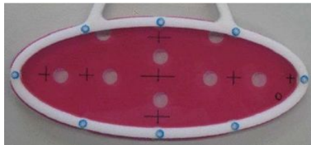
Figure 3.6: The muon stopping target in the MEG experiment mounted on a Rohacell frame [5].
