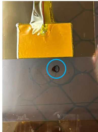
Figure 5.11: A deposit formed in the shifted irradiated position on the cathode. The other deposit in the first position had been removed.
