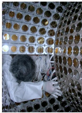
Figure 3.13: The LXe photon detector in MEG [15].
