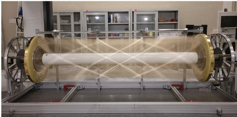
**Figure 2.10.** A picture of the entire drift chamber. The hyperbolic profile of the chamber is visible.
