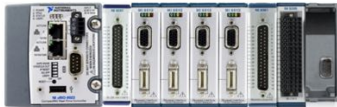
Figure 5.26: cRIO Controller with chassis and modules.
