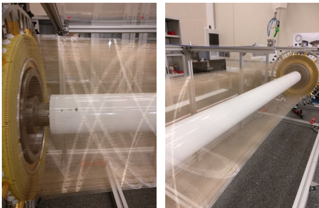
Figure 6.22: Detail of CDCHs with about 80% of the assembled layers
