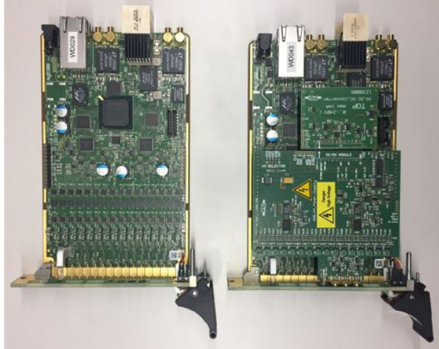
Figure 3.29: Left: The WaveDream Board with 16 single end channel. Right: The WaveDream Board with high voltage module installed.
