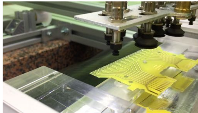
Figure 6.12: Wire PCB UP placed on the fixed structure.
