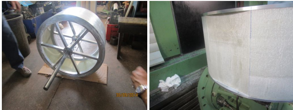
Figure 5.9: The cylinder in the different processing phases. The cylinder coupled with the spokes (Left). Finished cylinder (Right).
