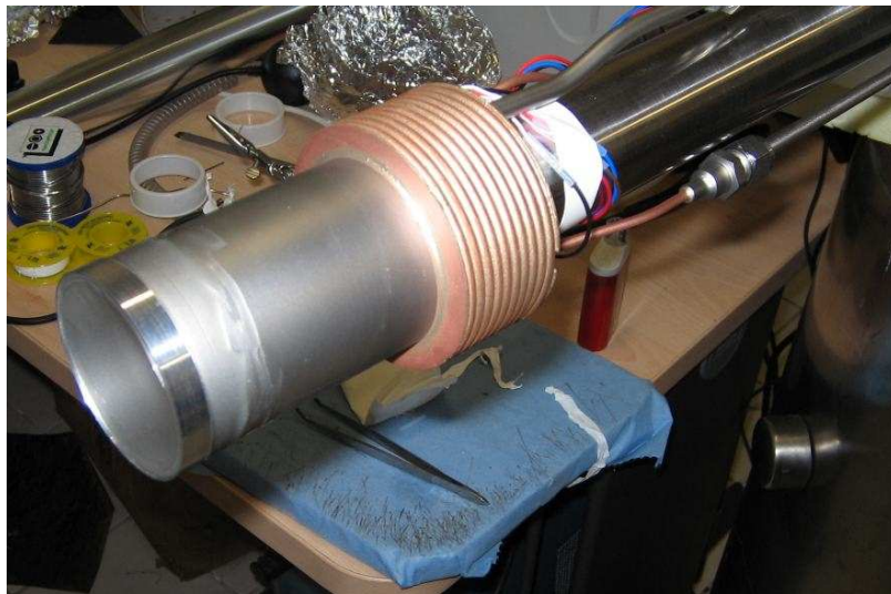
Figure 3.29: A picture of the \text{LH}_2 target cell for the pion charge exchange reaction before its installation
