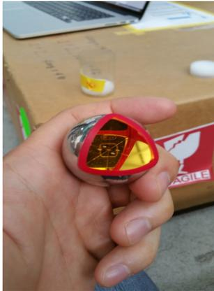
図 5.6: PSI 所有の反射鏡、Spherical mounted Retro-reflector (SMR)
