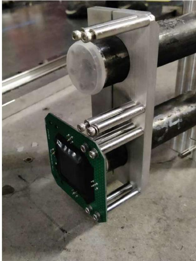
**Fig. 3.26:** One of the ToF detector prototypes fabricated in 2023 with four readout channels. The detector is mounted on the downstream detector module which is attached to the injection tubes.
