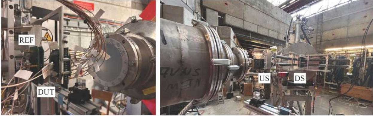
**Fig. 3.31:** The *short* and *long* configurations, used to extract the main parameters of the TOF detectors.
