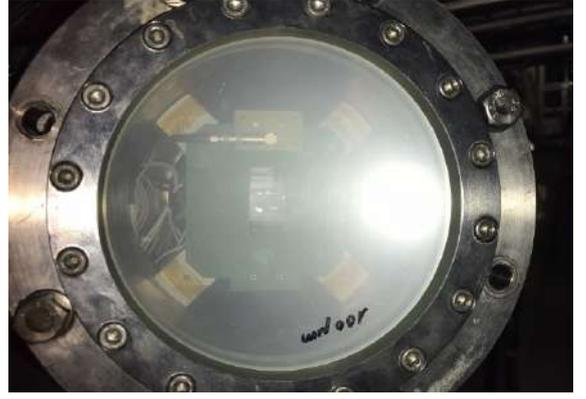
(b) The view of the detectors from the Mylar window before making it light-tight.
