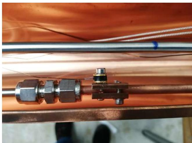
(a) The sensor placed on the He lines with a Cu 'clamp'.
