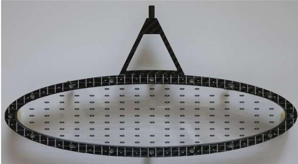
**Fig. 5.14:** Picture of the BC400 target. Clearly visible is the dot pattern on both the target and carbon fiber frame. Six holes, admittedly less visible, are located on the axes of the ellipse.
