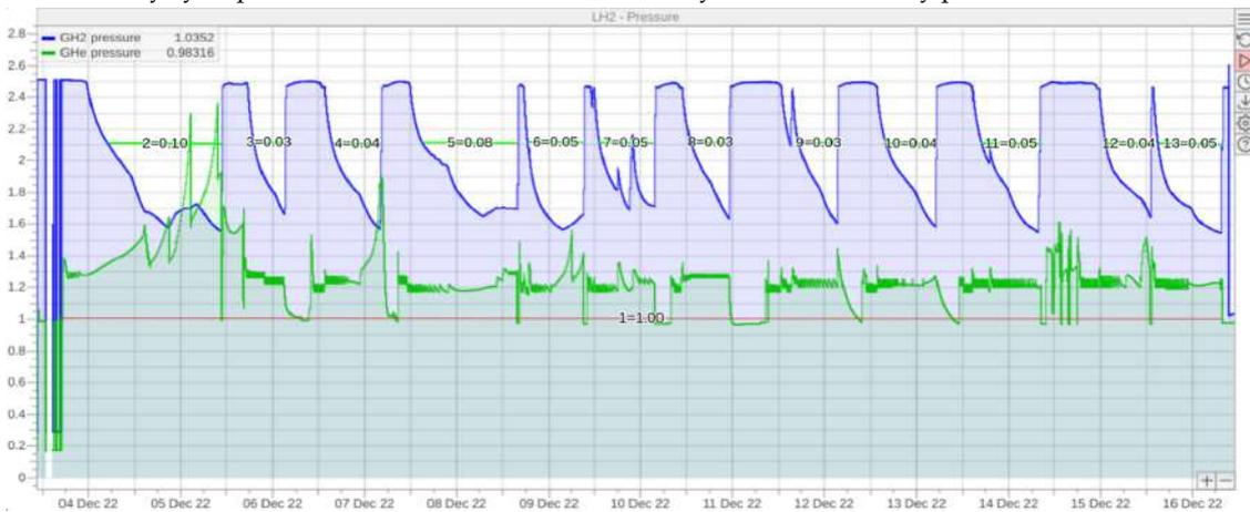
(b) CEX 2022: beam below 2.1 bar. This translates to a duty cycle of  $D_{2022} \approx 0.6$ , with target level  $> 50\%$ .
