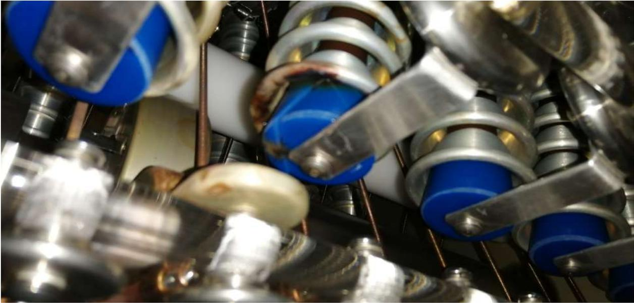
(a) Discovery of the burning marks on two rectifiers. The reflectivity was a challenge in taking the picture.
