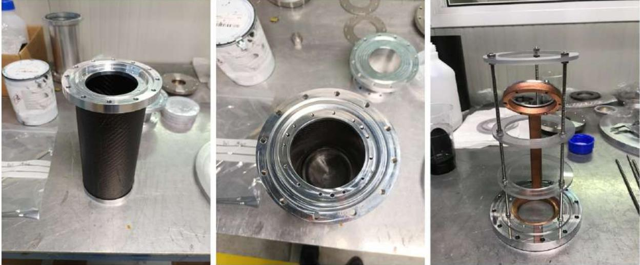
**Fig. 7.4:** Construction of the carbon fiber vacuum chamber and picture of the copper arm used to hold the targets and of the internal structure of the chamber.
