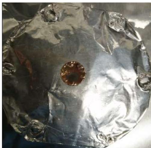
**Fig. 7.26:** Here is a picture of the target itself after two days of data-taking at 5 and 10  $\mu\text{A}$ . The dark spot marks the position on which the beam was impinging.
