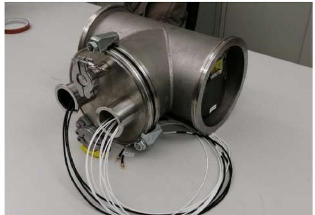
(b) "T" beamline piece used as vacuum chamber.
