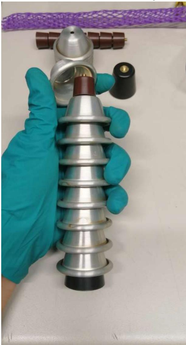
(b) Assembly of one of the new stack: black - resistors; brown - diodes; metallic - aluminum capacitors.
