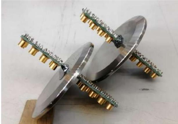
(a) Custom feed-throughs: PCB board, with soldered connectors, sealed with Stycast in a blind flange.
