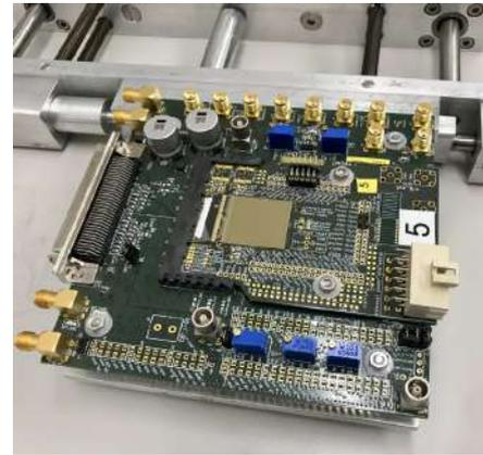
(b) Picture of one of the MuPix10 mounted on the two PCBs.
