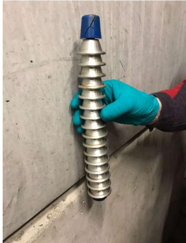
(c) Broken rectifier ass'y after the extraction: clearly visible is the burned blue resistor at the top.
