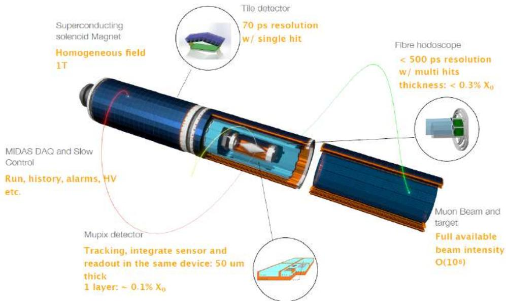
Fig. 1.2: Pictorial view of the Mu3e apparatus [25].
