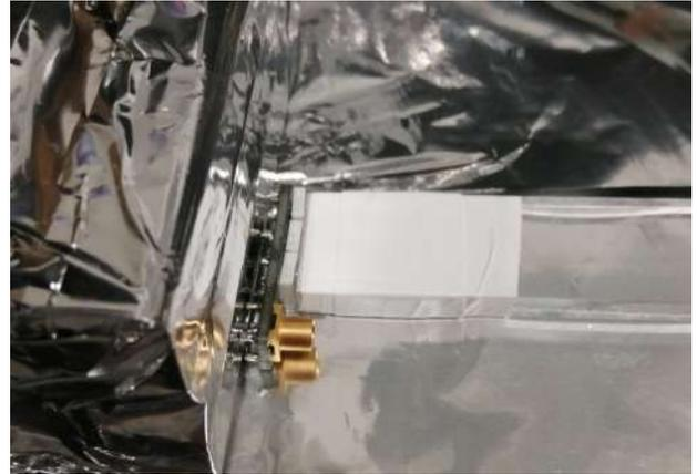
(b) A small PCB board with 3 SiPMs and one connector attached with optical cement to one of the scintillators.
