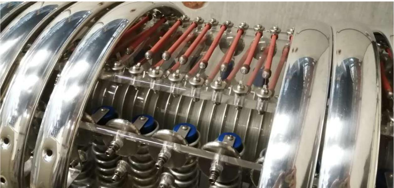
Fig. 5.23: Top view of the CW after the removal of a few *corona rings*. Here we can see all the elements of a CW circuit: red - the resistors on top; metallic rings on the central tube - the capacitors; blue and metallic cups - the resistance and capacitors of the rectifiers, which run vertically.
