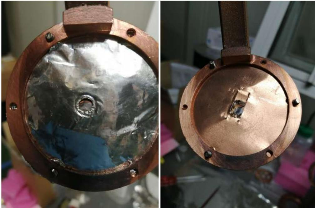
**Fig. 7.25:** Two different ways to hold the small LiPON sample given to us by the PSI colleagues. We first tried to hold it in place with folded aluminum foils. We later realized this was not the optimal solution given the spectrum produced by protons on Al. We then moved to a cleaner Cu setup.
