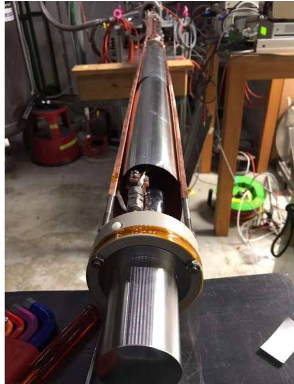
(c) Shieldig was added around the whole structure.
