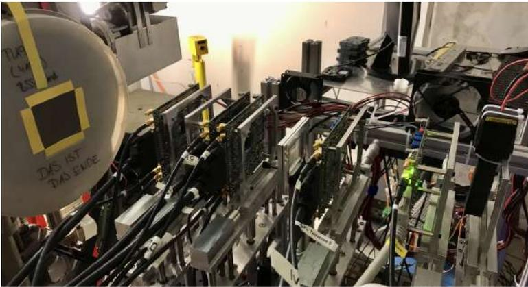
(a) Picture of the setup for the beamtime of 2021. On the right, the scintillator was used as an external trigger, on the left, beam exit window.
