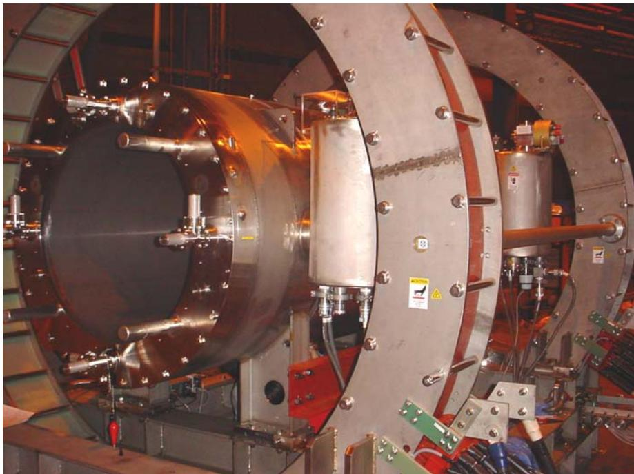
**Figure 2.8:** The COBRA magnet. Two large coils around the main magnet are to compensate and suppress the magnetic field at the LXe detector.
