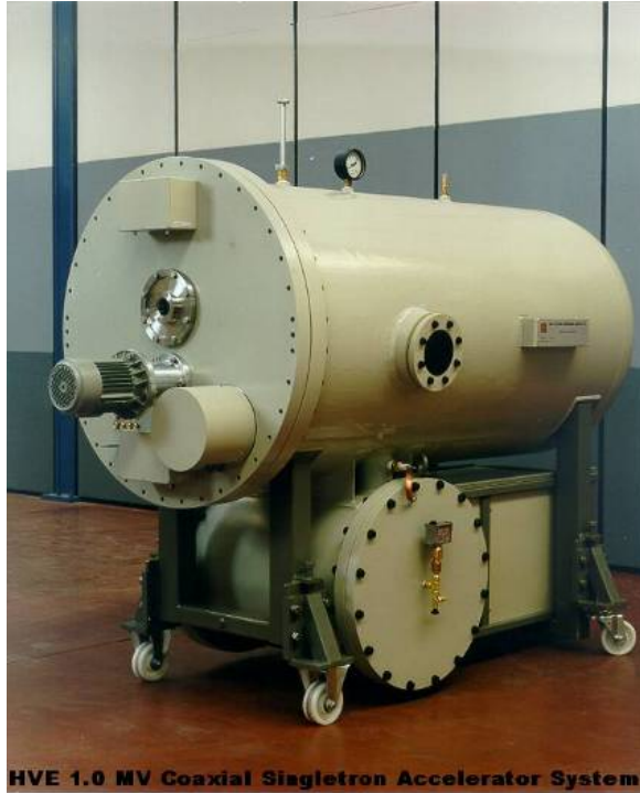
Figure 3.41: 1 MeV Cockcroft-Walton proton accelerator.
