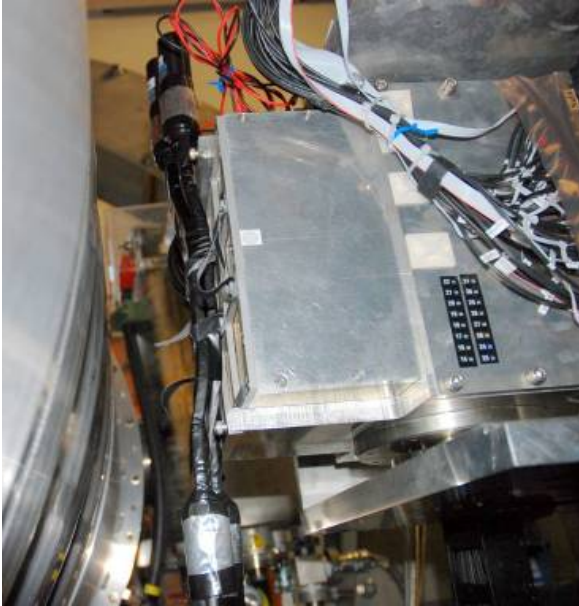
Figure 3.39: Picture of the NaI detector. It consists of a lead converter, two plastic scintillators, and nine NaI crystals.
