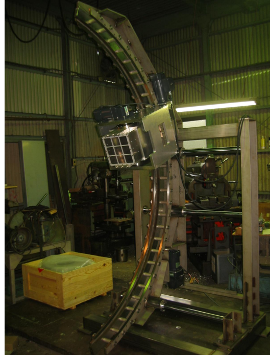
Figure 3.40: Movable stage of the NaI detector to be placed at the opposite side of the LXe gamma-ray detector.
