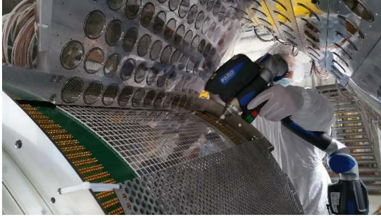
Figure 5.3: (Left) The surface of the MPPCs is scanned with the laser scanner [48]. (Right) An example of the measured height (perpendicular to the surface) distribution. The MPPC package structure (hosting four chips) is visible.
