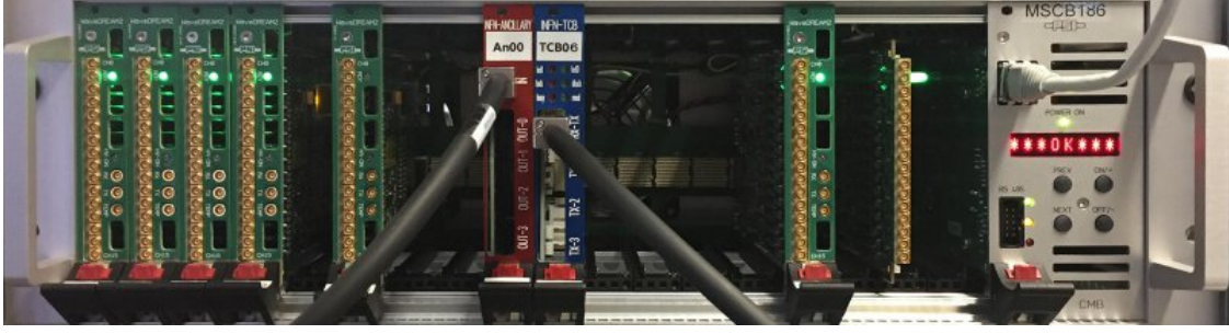
Figure 2.31: A WaveDREAM crate [34].
