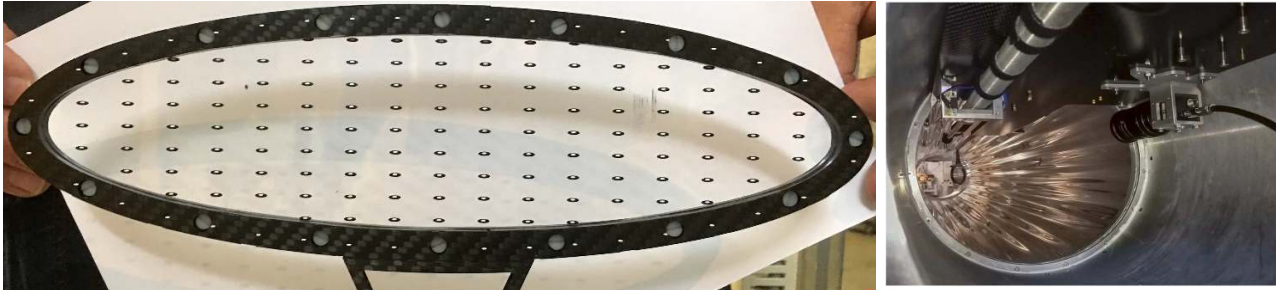
Figure 2.4: Muon stopping target for the MEG II experiment and a CCD monitoring camera [34, 61]. When projected in the global XY plane of the MEG II experiment, the ellipse shape results in a circle.
