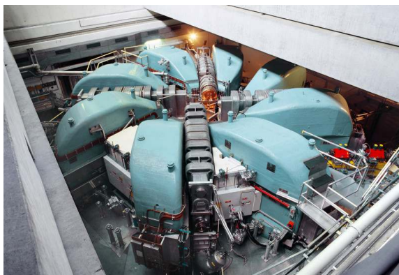
Figure 2.3: The main proton accelerator at PSI [60].
