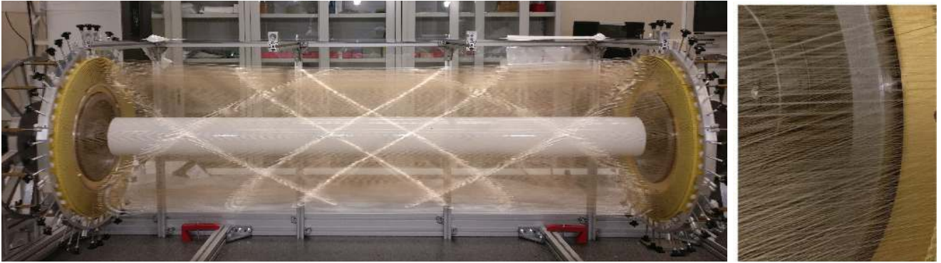
Figure 2.8: Pictures of CDCH taken before the enclosure by the carbon support frame [34]. Left: Full picture of the entire drift chamber. The hyperbolic shape is visible. Right: A zoom-up picture showing the wire crossing in the stereo geometry.
