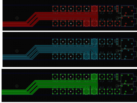
Figure 4.57: Three layers of top (red), inner (blue), and bottom (green) layers.
