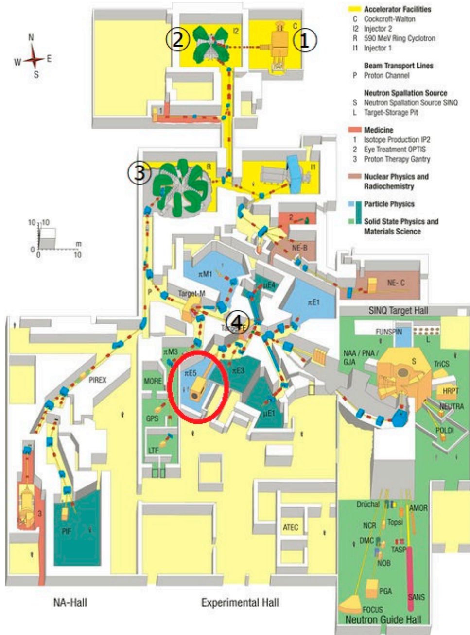
Figure 3.8: Overview of Beamlines in PSI. (1) Cockcroft-Wolton injector. (2) Injector. (3) 590 MeV Ring Cyclotron. (4) Target E. \pi E5 area is encircled in red.
