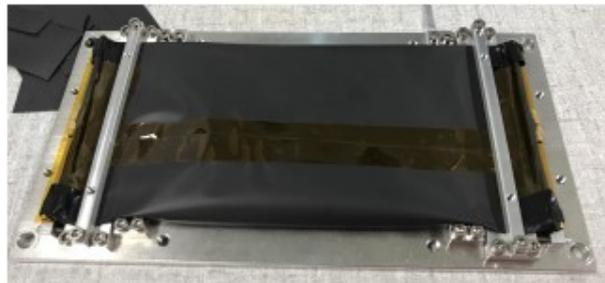
Figure 2.45: Pre-shower counter module [56]. A fast plastic scintillator is wrapped with reflectors of aluminized mylar and then shielded by a black sheet. The scintillator is read out by 16 MPPCs at both ends.
