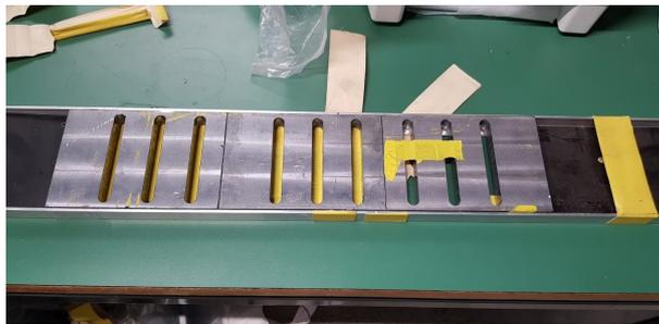
Figure 6.6: Collimator for the position resolution measurement in the MEG experiment.
