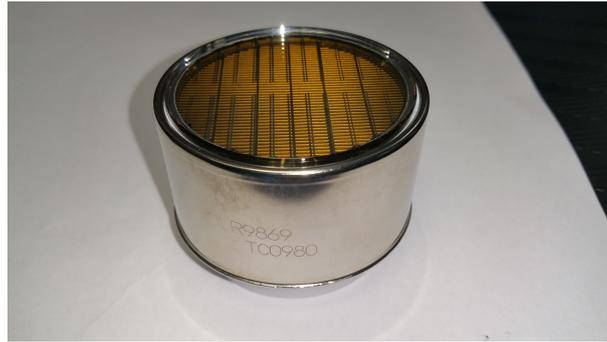
Figure 2.16: VUV-sensitive PMT for MEG (II) (R9869).
