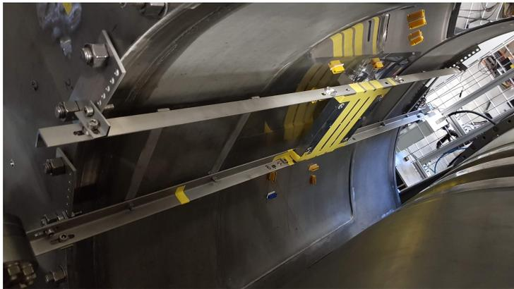
Figure 6.9: Installed collimator between the COBRA and the detector. The collimator was fixed by screws and tapes to the support structure, and the support structure was fixed to the lateral flanges of the detector by screws.
