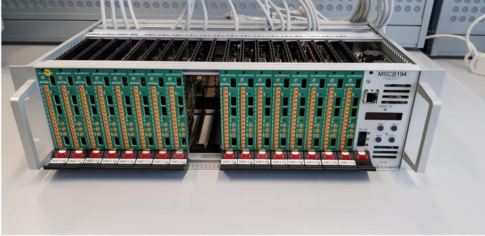
Figure 2.50: WaveDREAM boards in a crate. A WaveDREAM crate has 16 slots for WaveDREAM boards and two slots for a DCB and a TCB.
