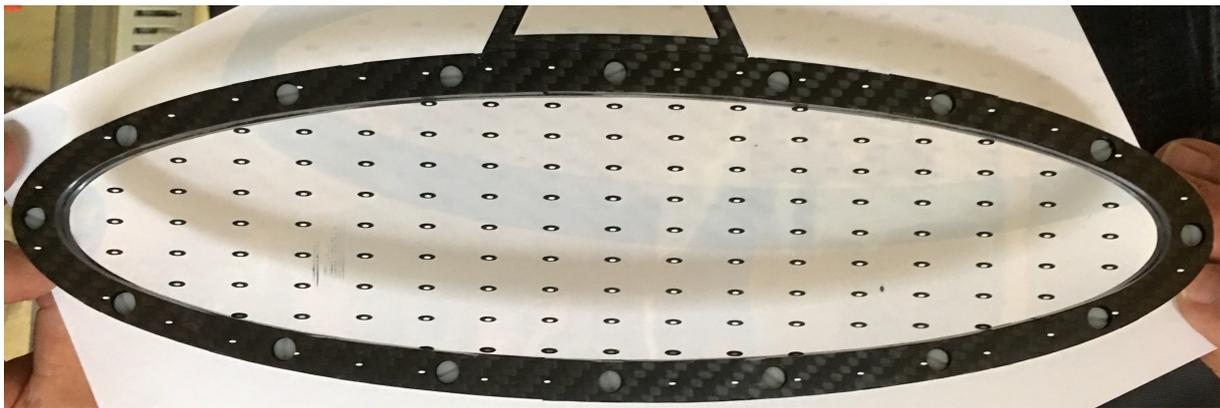
Figure 2.3: Muon stopping target for the MEG II experiment [29]. An ellipse plastic film of  $174\ \mu\text{m}$  thick with holes is supported by a rigid carbon-fiber frame of  $200\ \mu\text{m}$  thick.
