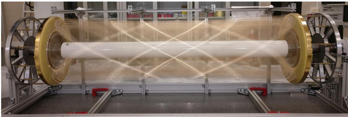
Figure 2.10: Drift chamber with all wires [29].
