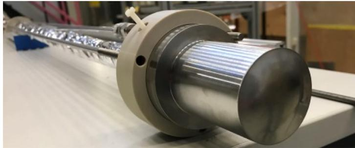
Figure 2.43: Cell of the LH<sub>2</sub> target used in the 2021  $\pi^0$  run.
