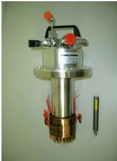
(a) Pulse tube refrigerator for LXe detector
