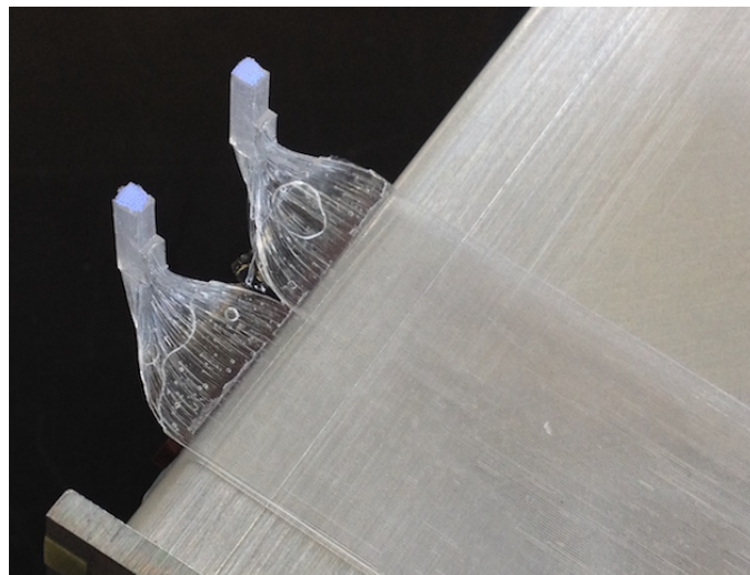
Figure 3.21: Prototype of the bundled fibers (64 fibers \times 2).
