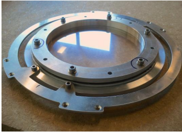
Figure 6.1: RDC mockup ( 230\text{ }\mu\text{m} thick Mylar foil).
