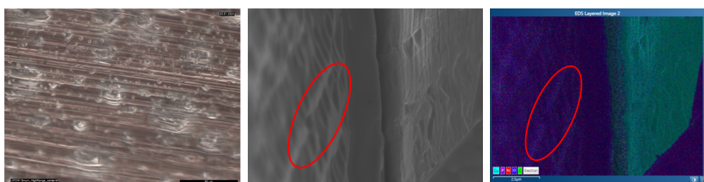
Figure 4.17: Optical microscope (left), SEM (middle) and EDX (right) images of the 2024 1.9 \mu\text{m} -thick LiPON surface. The red ellipse corresponds to the same region on the two right pictures and surrounds bump-like structures on the deposit surface.
