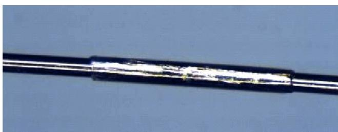
**Figure 6.2:** Closeup of  $^{241}\text{Am}$  source on wire. Diameter is  $100\ \mu\text{m}$  and length is about 2 mm.
