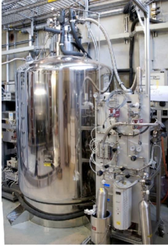
**Figure 3.18:** Liquid xenon tank and gaseous purification system.
