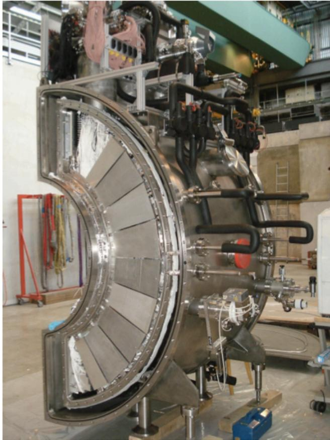
**Figure 3.15:** Liquid xenon detector
