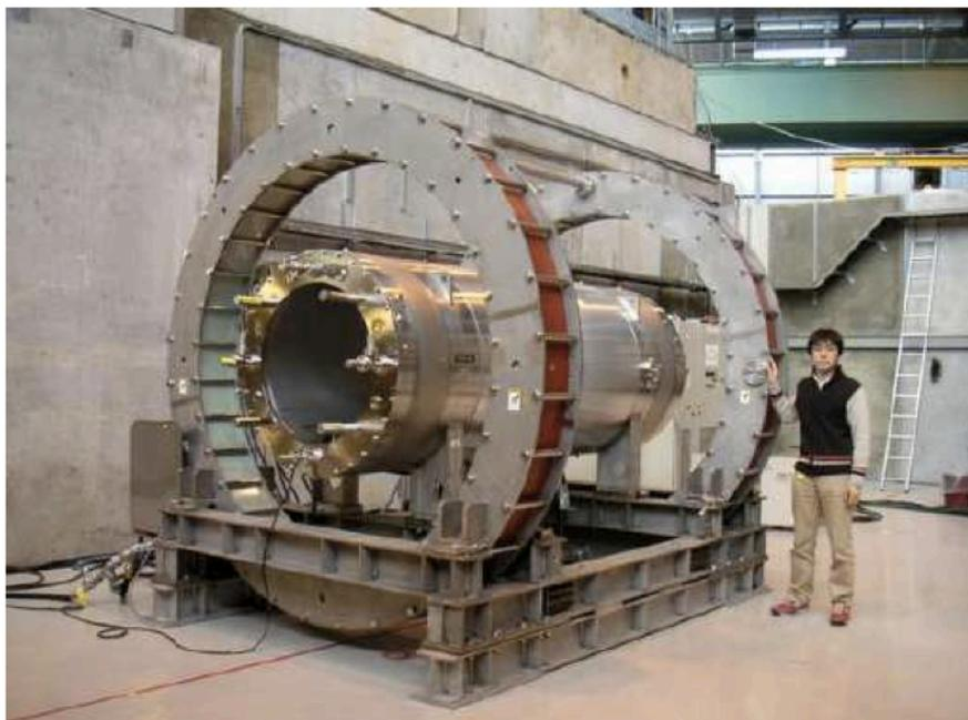
**Figure 3.20:** A photograph of COBRA magnet.
