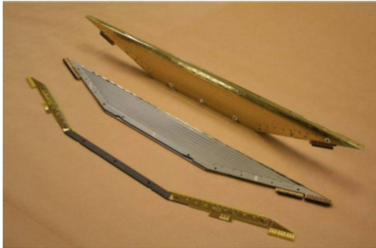
**Figure 3.26:** Drift chamber module.
