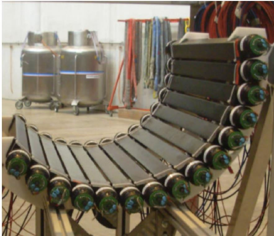
**Figure 3.30:** Picture of timing  $\phi$ -counter.
