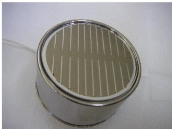
**Figure 3.12:** PMT for the LXe detector.
