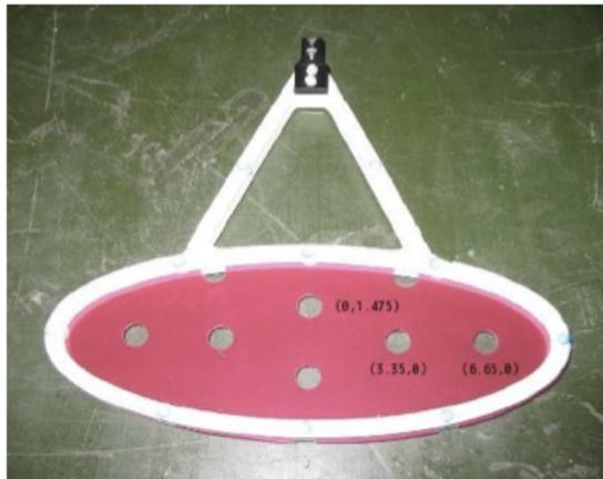
**Figure 3.8:** Muon stopping target.
