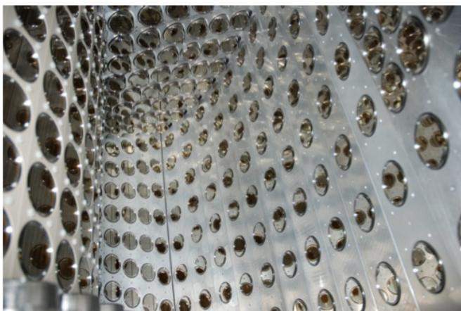
**Figure 3.16:** PMTs mounted inside the LXe detector.
