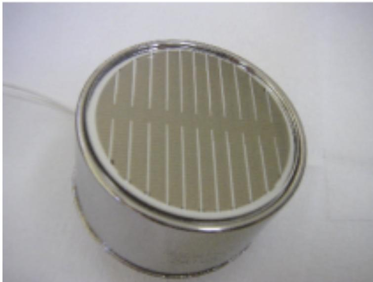
Figure 2.13: Hamamatsu R9288. Aluminum strips are attached on the surface of cathode to avoid increasing of surface resistance in low temperature.
