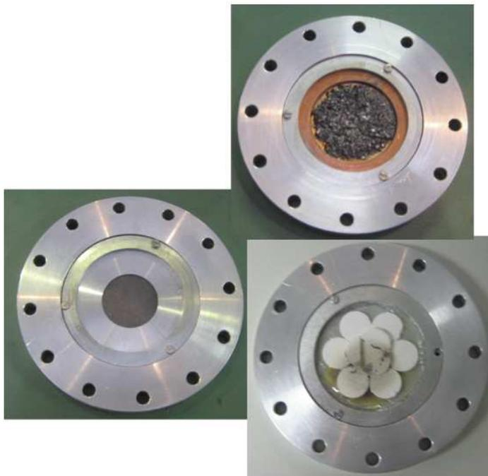
Figure 13.6: *The different boron targets. Upper target: pure boron. Lower targets, left: boron carbide  $B_4C$ , right: lithium tetraborate  $Li_2B_4O_7$ .*
