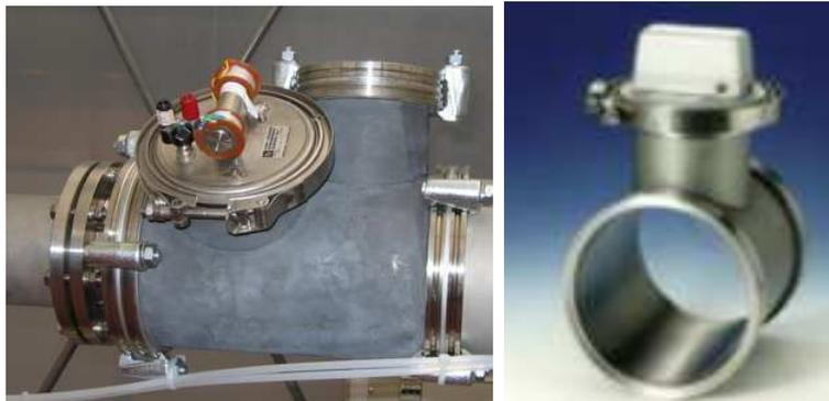
Figure 10.21: *Closed and open wire scanner.*
