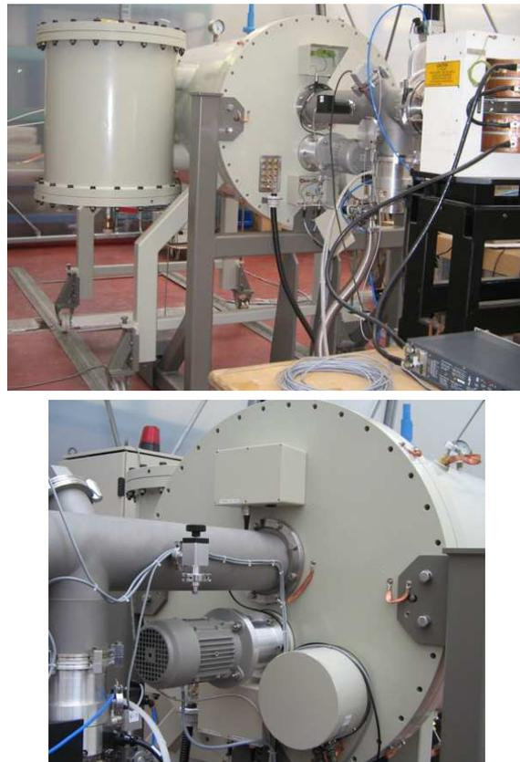
Figure 10.13: *A view of the C-W accelerator (left). A detail of the C-W front-face (right).*
