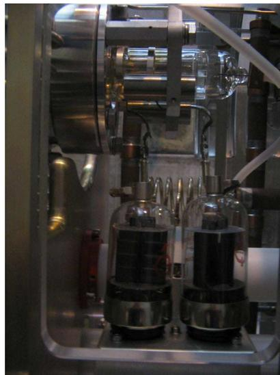
Figure 10.15: The RF ion source.
