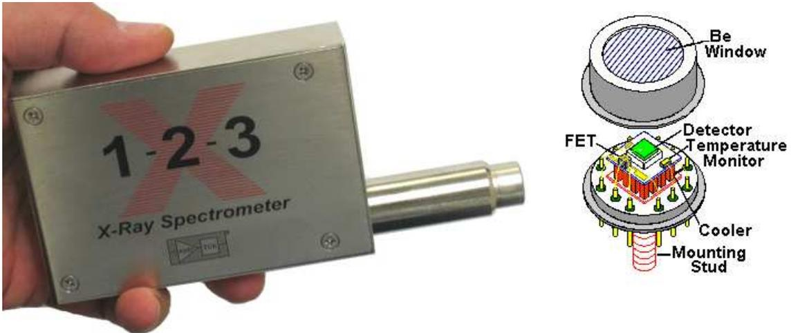
Figure 14.7: The X-ray Si-pin detector.
