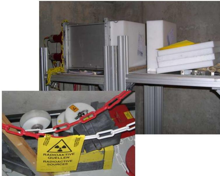
Figure 9.8: *The experimental set-up for the test of the 9 MeV  $\gamma$ -generator. A large NaI detector was used.*
