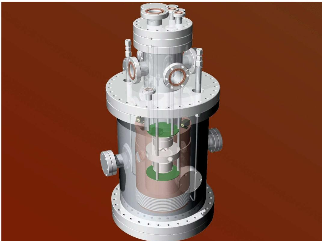
Figure 5.10: A detail of the small cryostat in Pisa. One can see the internal volume, where the two PMTs are immersed. The reference PMT is mounted at the bottom of the cryostat, the PMT under test is in front of it, at the top of the cryostat.
