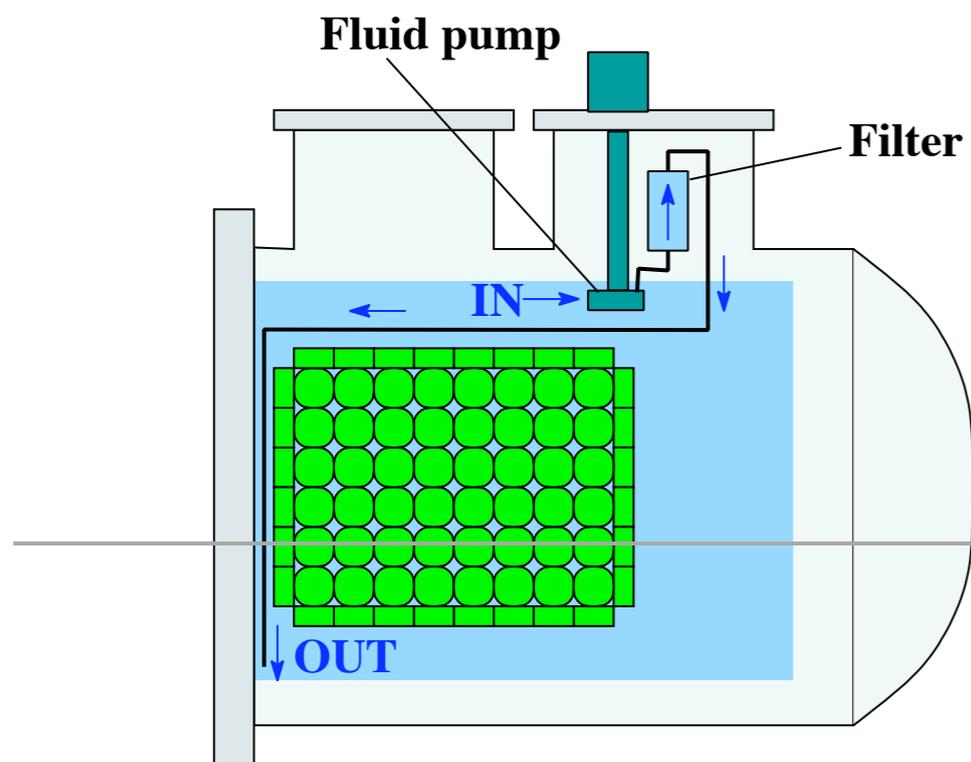
Purification system installed in 100L prototype
