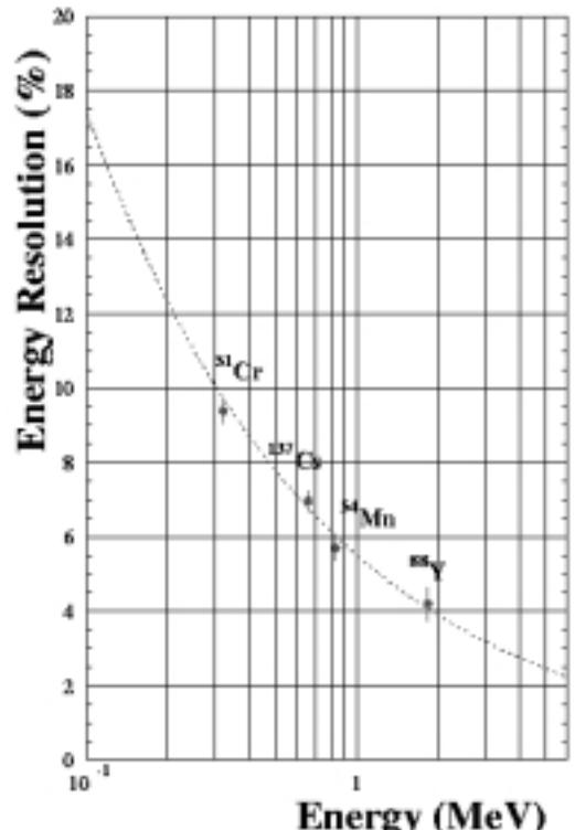
Figure 3: Energy resolution measured with gamma-ray sources as compared to the predictions (dashed line) by the simulation.
