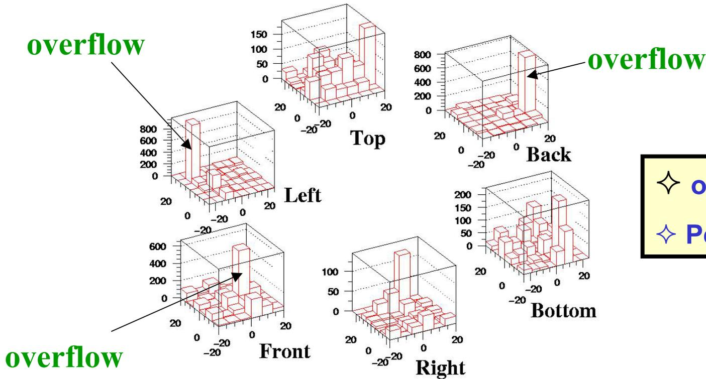
Some broken amps on an ADC caused heavy damage to many amps on all ADCs.
