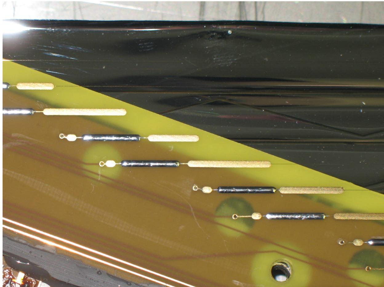
2) The potting glue for the HV protection was inadequate: change on all chamber to epoxy glue
