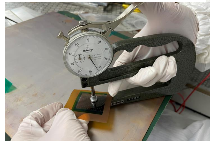
Measurement of pillar heights
