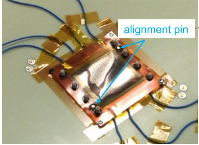
Electrodes are fixed by alignment pins at the edges
