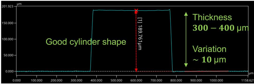
\*same material on the previous electrode but ~190  $\mu\text{m}$  thickness
