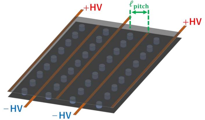
Voltage drop ( $\rho_S = 10 \text{ M}\Omega/\text{sq}$ )
