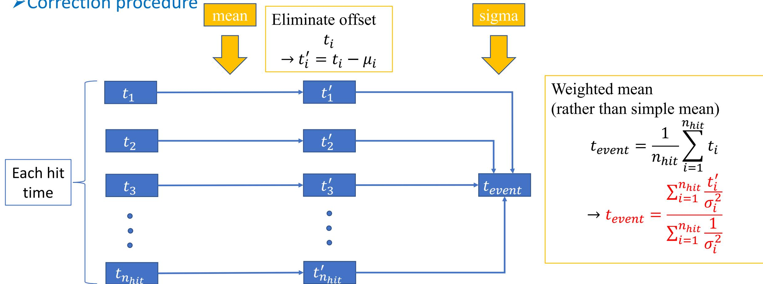
Remaining position dependence can be made use of when combining each hit time to obtain total positron time
