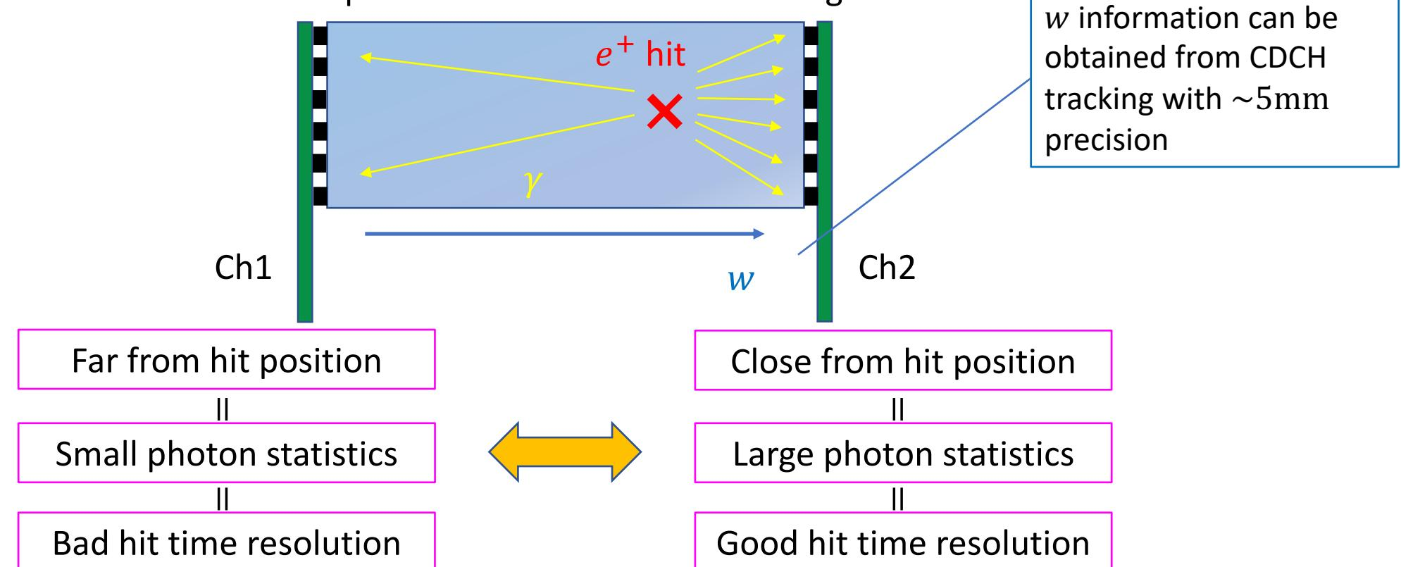
This dependence can be made use of when combining each channel time to obtain hit time
