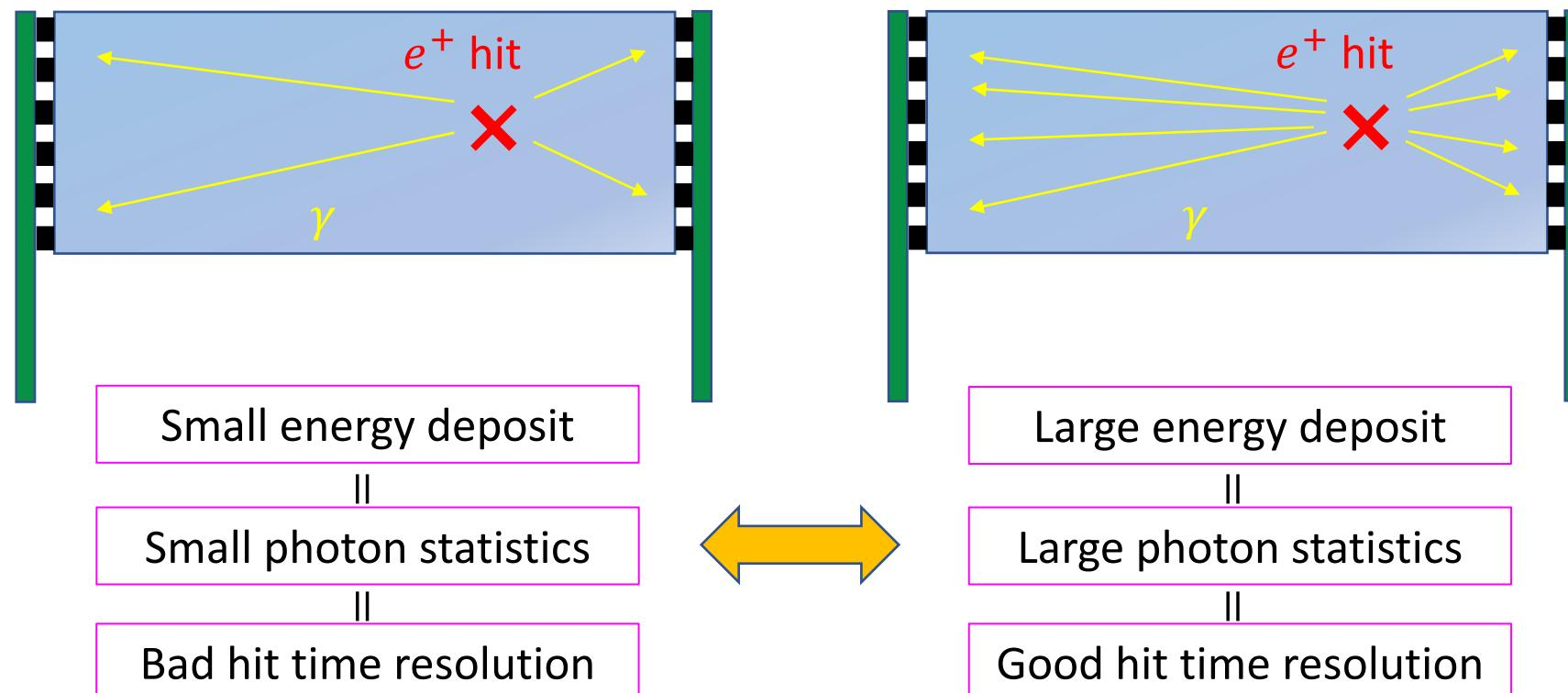
This dependence can be made use of when combining each hit time to obtain total positron time
