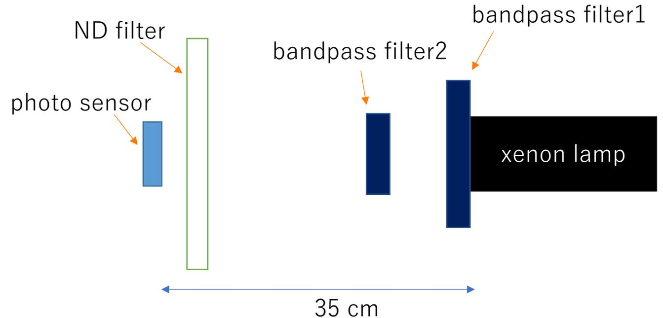
Light from the xenon lamp enters after passing through filters.
