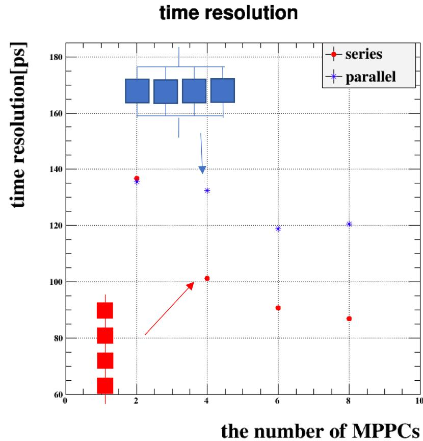
Checked difference between series and parallel connection. Resolution of series connection is superior to that of parallel as expected.
