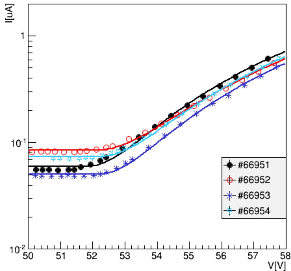
MPPCs connected in series or parallel must have similar characteristics.
