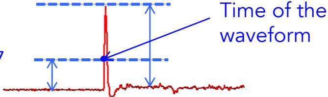
Hit time ( $t_{hit}$ ) is calculated by averaging both ends.
