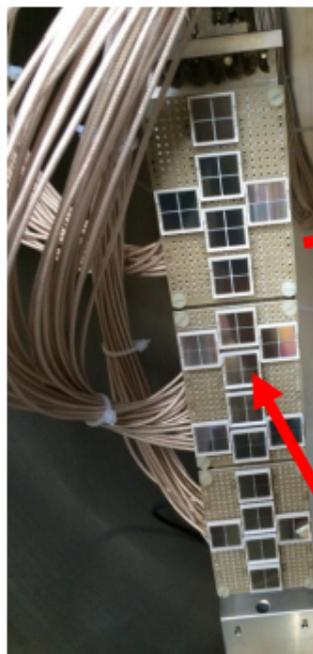
No protection windows on MPPCs to avoid refraction in gaseous xenon
