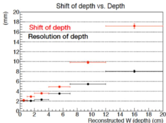
shift of depth > resolution of depth → significant bias
