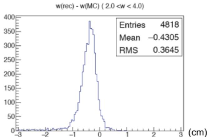
distribution of the difference between real conversion depth and reconstructed depth (simulation)
