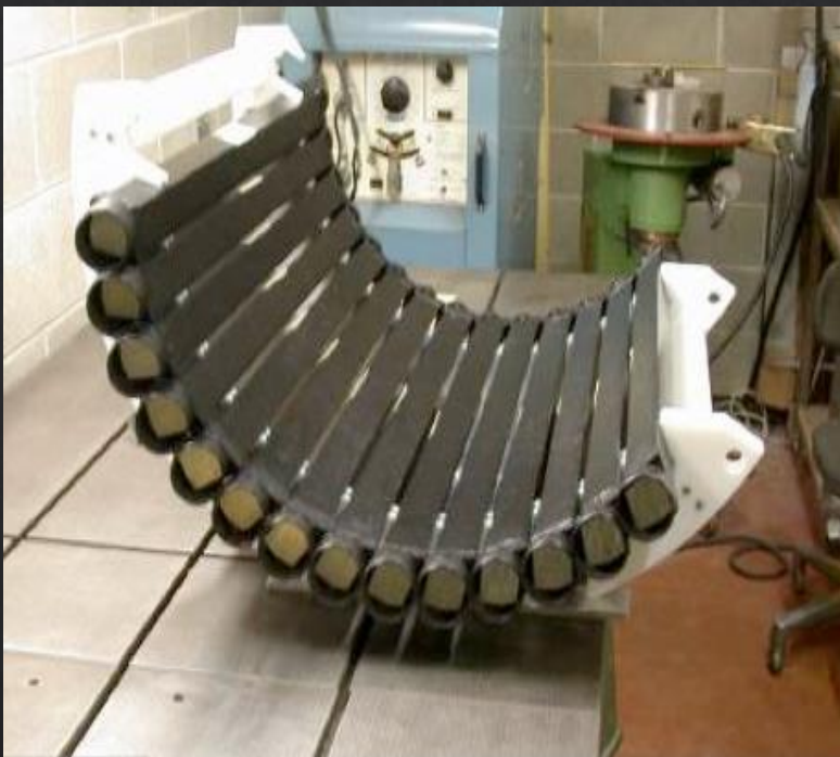
Assembled \phi counter (one of two)
