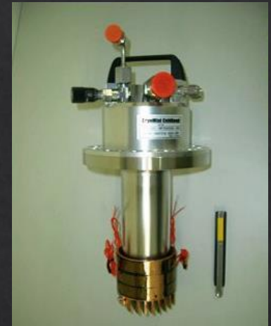
200 W pulse tube refrigerator
