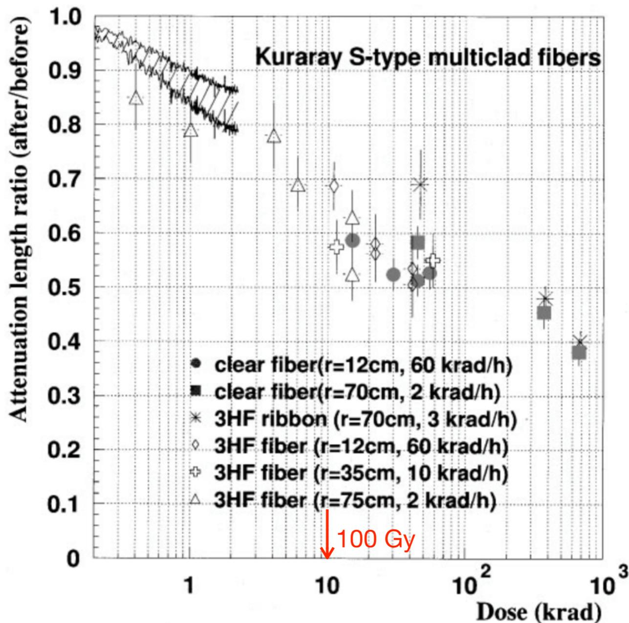
3HF fiber : Scintillating fiber with wavelength shifter for radiation hardness
