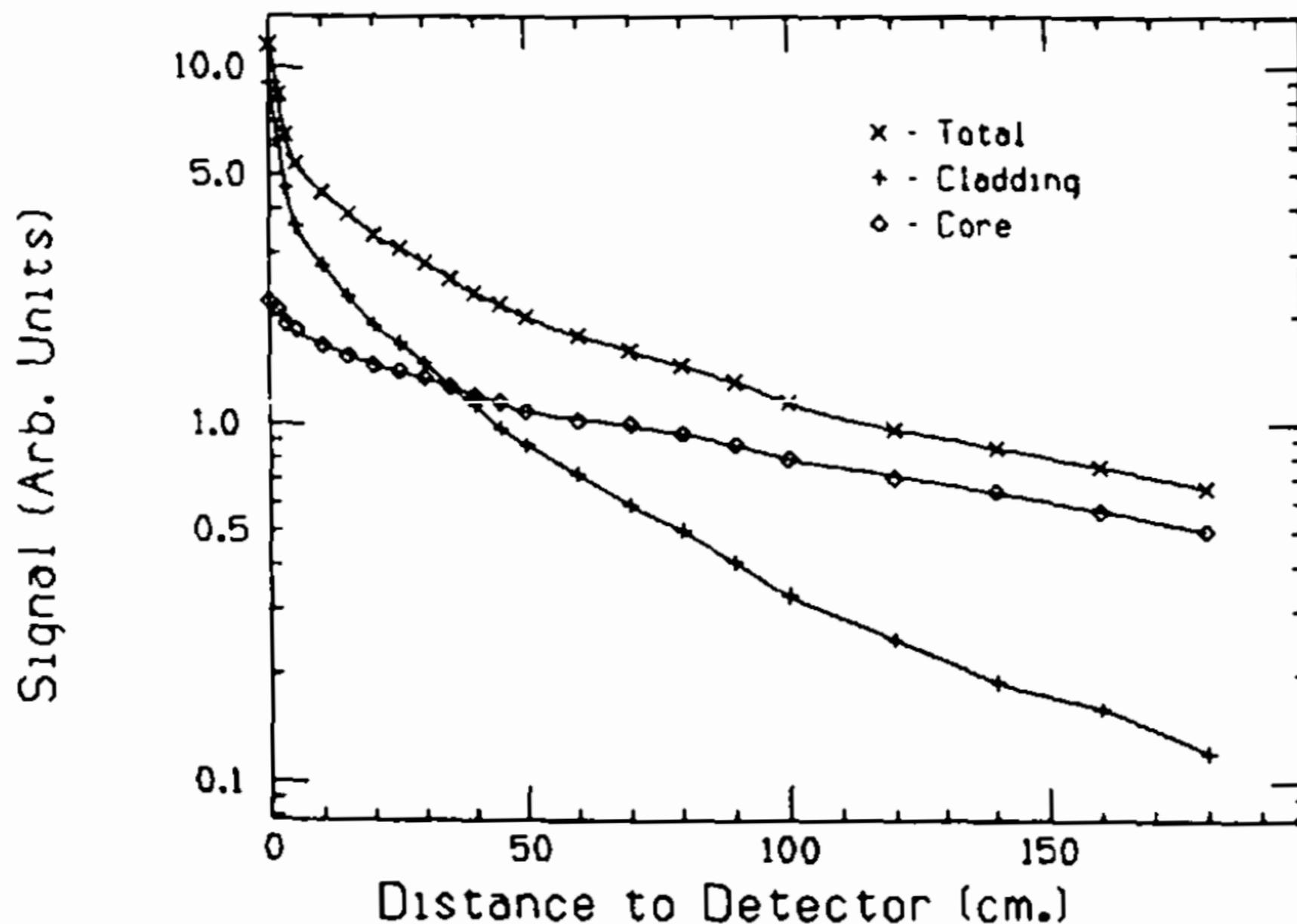
Fig. 13. Attenuation length curves for "core," "cladding," and "core + cladding" light.
