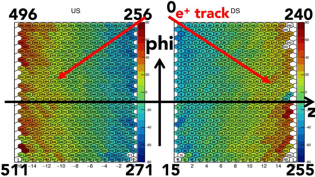
↓ Calculated time offset – true time offset / ↑ its position dependence
