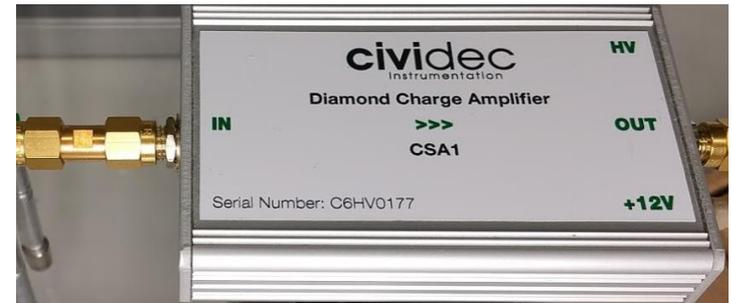
High gain, low noise charge amplifier (CIVIDEC C6HV0177), 5.7 mV/fC,
