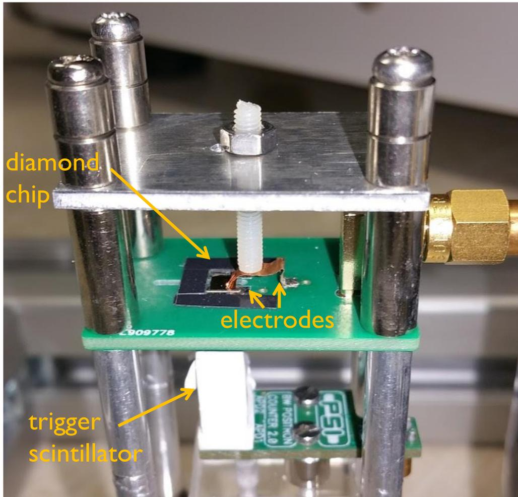
We tested diamond samples with radioactive sources placed on diamond.
