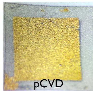
Au (200nm) on both sides as electrodes
