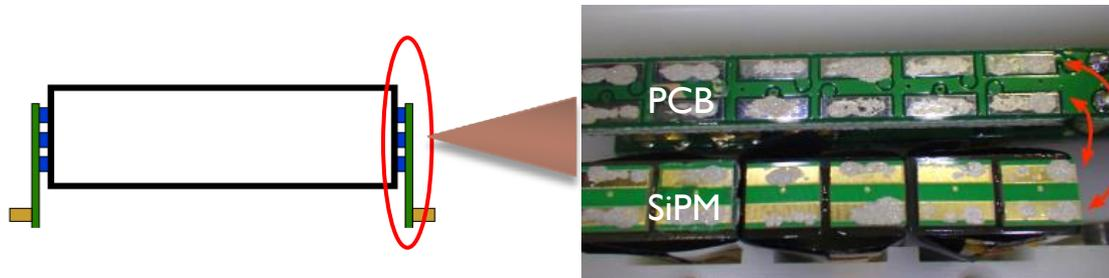
We used conductive epoxy instead of soldering to avoid heat damage
