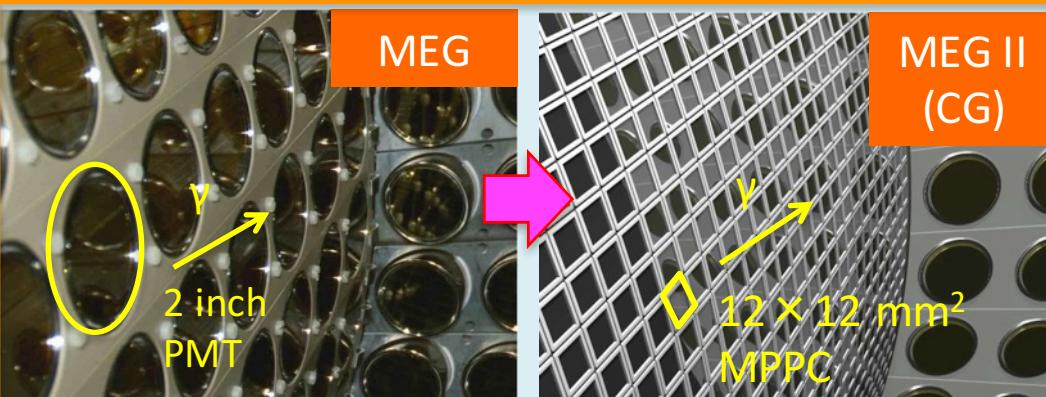
We will replace 216 2-inch PMTs on the  $\gamma$ -entrance face with 4092  $12 \times 12 \text{ mm}^2$  MPPCs.
