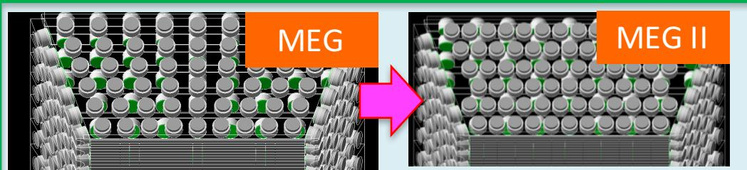
Number of PMT increases ( $54 \rightarrow 73$ ) and PMT is placed staggered
