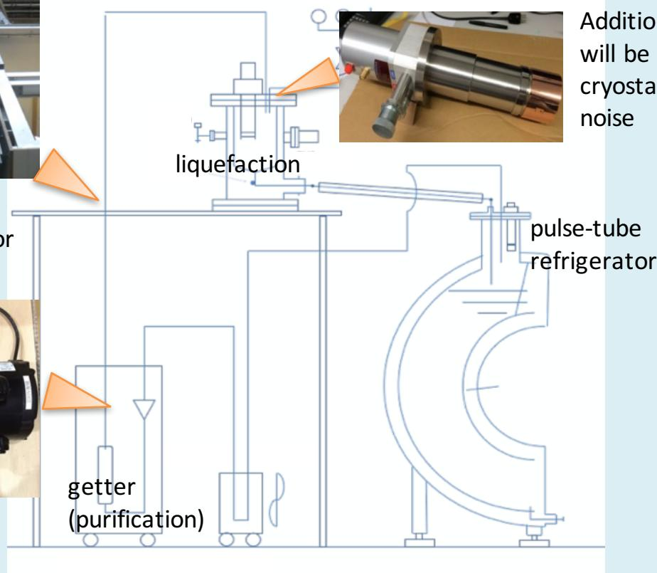
Additional GM refrigerator will be placed far from cryostat to prevent from noise
