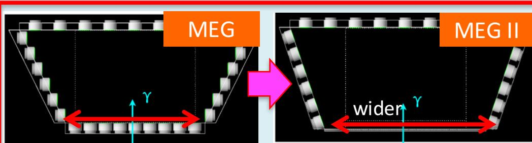
Different PMT angle of lateral face
