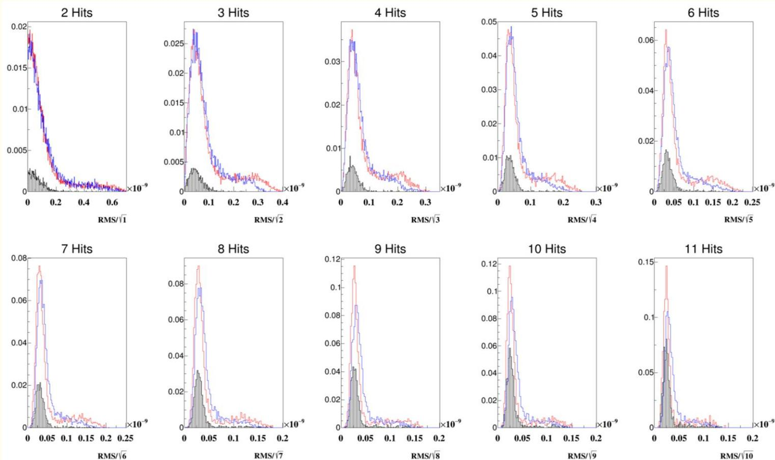
Resolutions of 28.5 ps (MC), 31.1 ps (Data) at  $n \text{ hits} = 8$ .
