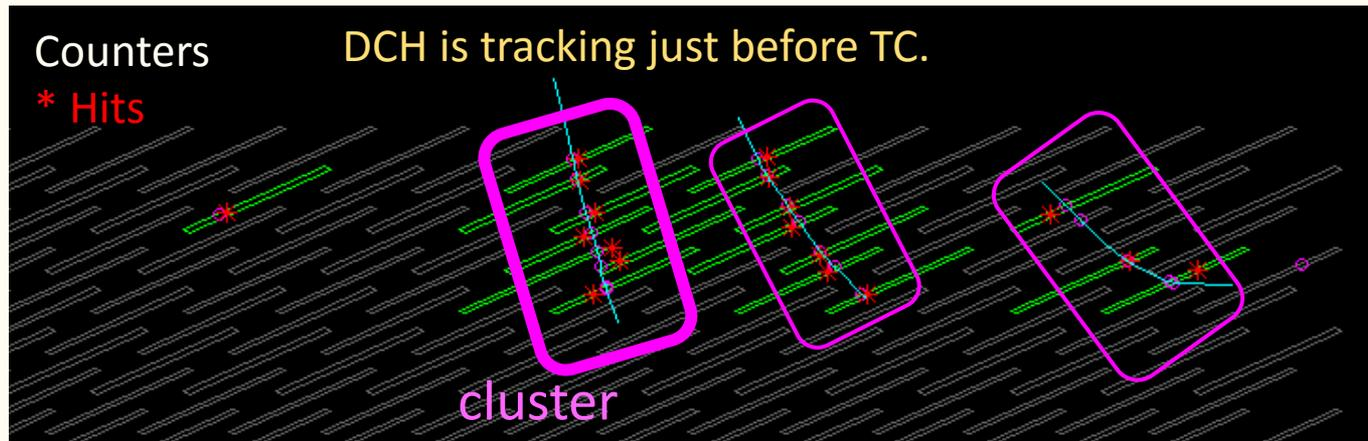
All hits from the same track and the same turn should be included in a cluster. Following parameters should be checked.
