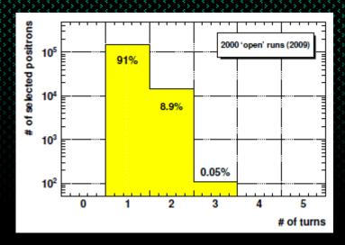
Sometimes positron runs more than 1 turns before exit drift chamber.
