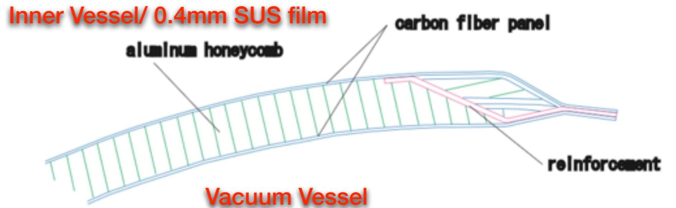
Figure 7. Cross section of transition area of carbon-fiber honeycomb panel.
