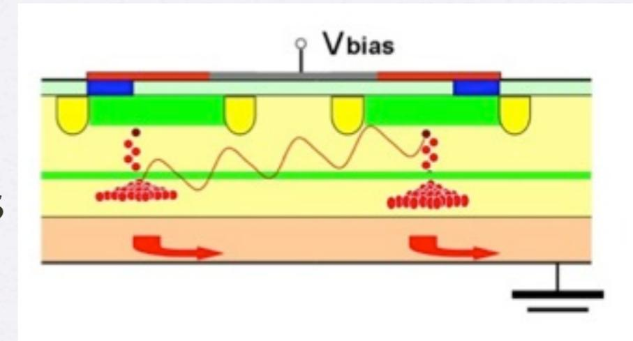
Inter-pixel groove to block  $\gamma$
