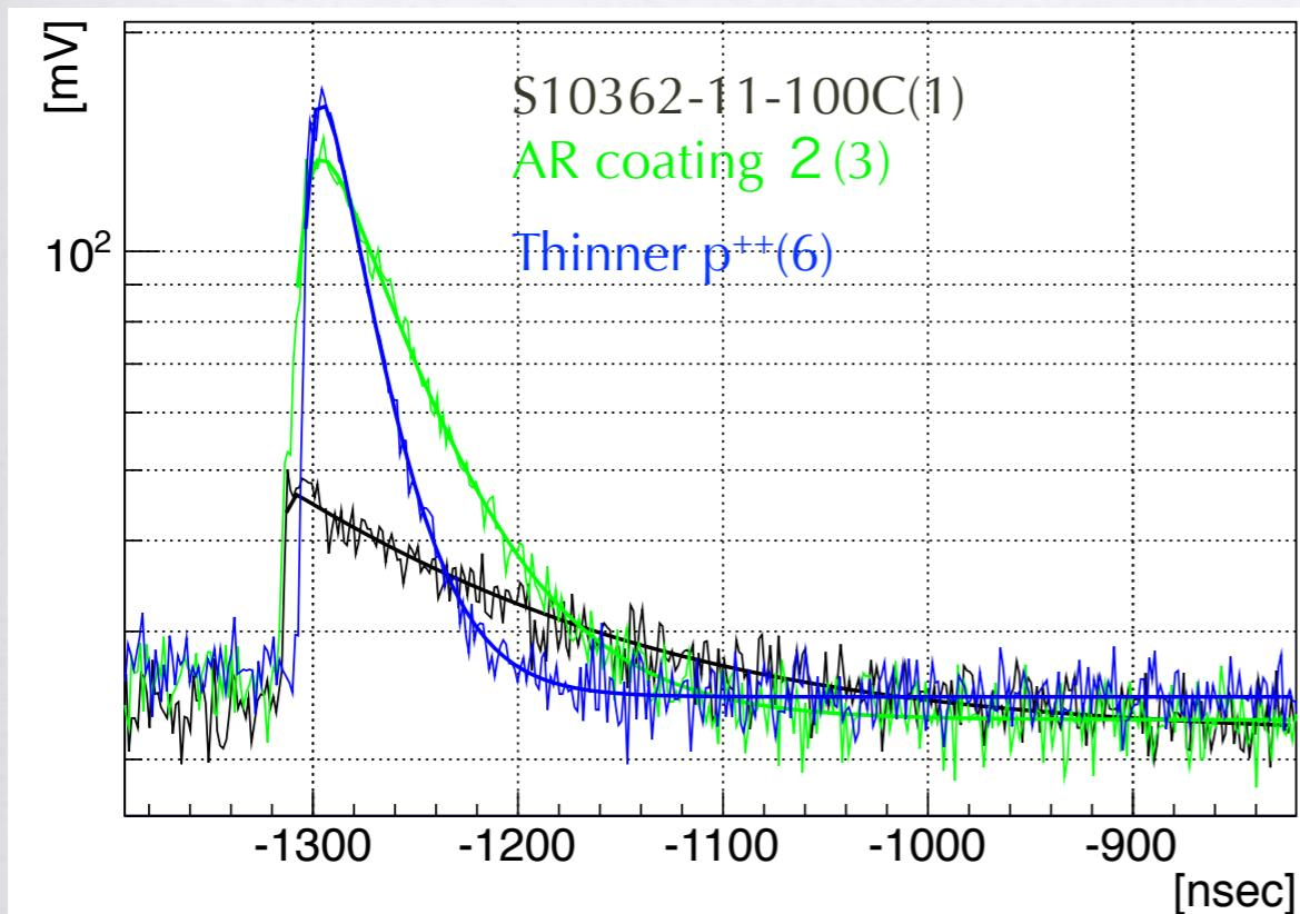
S10362-33-100C : long tail by 100μm pitch (large C)
