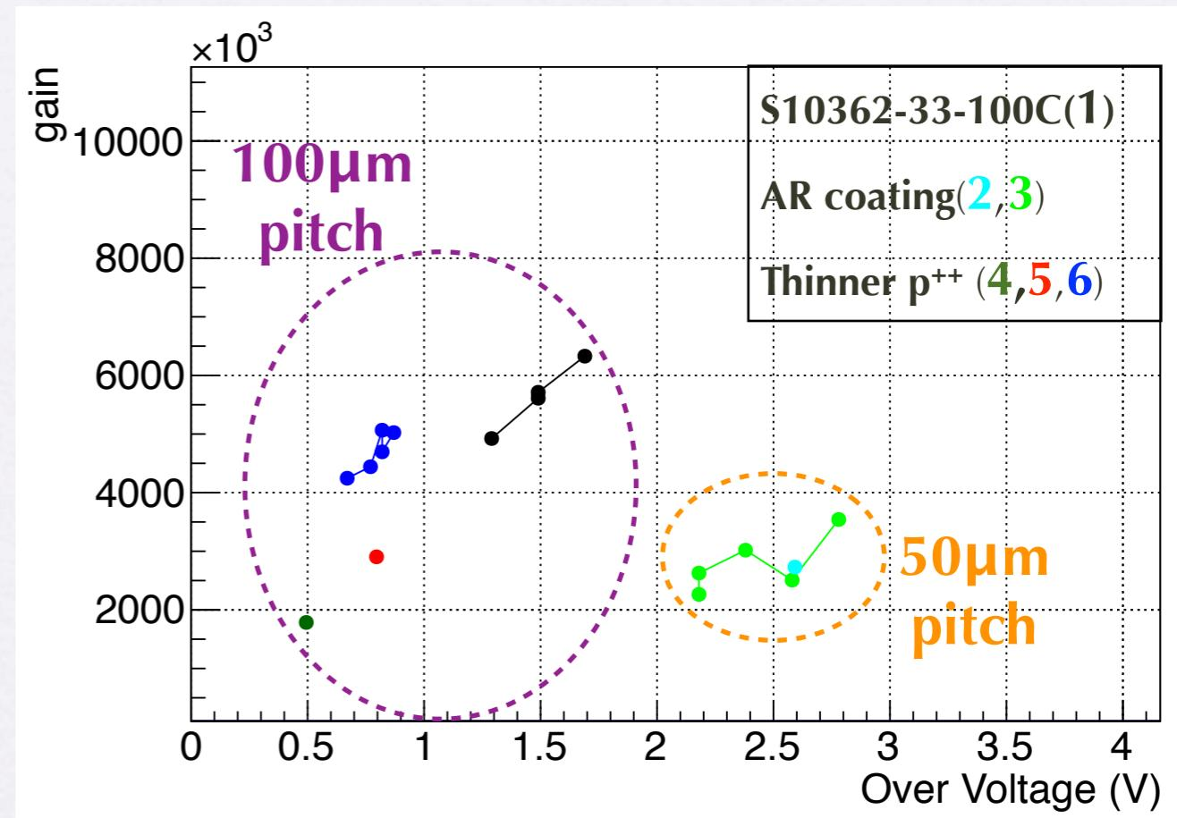
Pixel capacitance depends on the pixel pitch size
