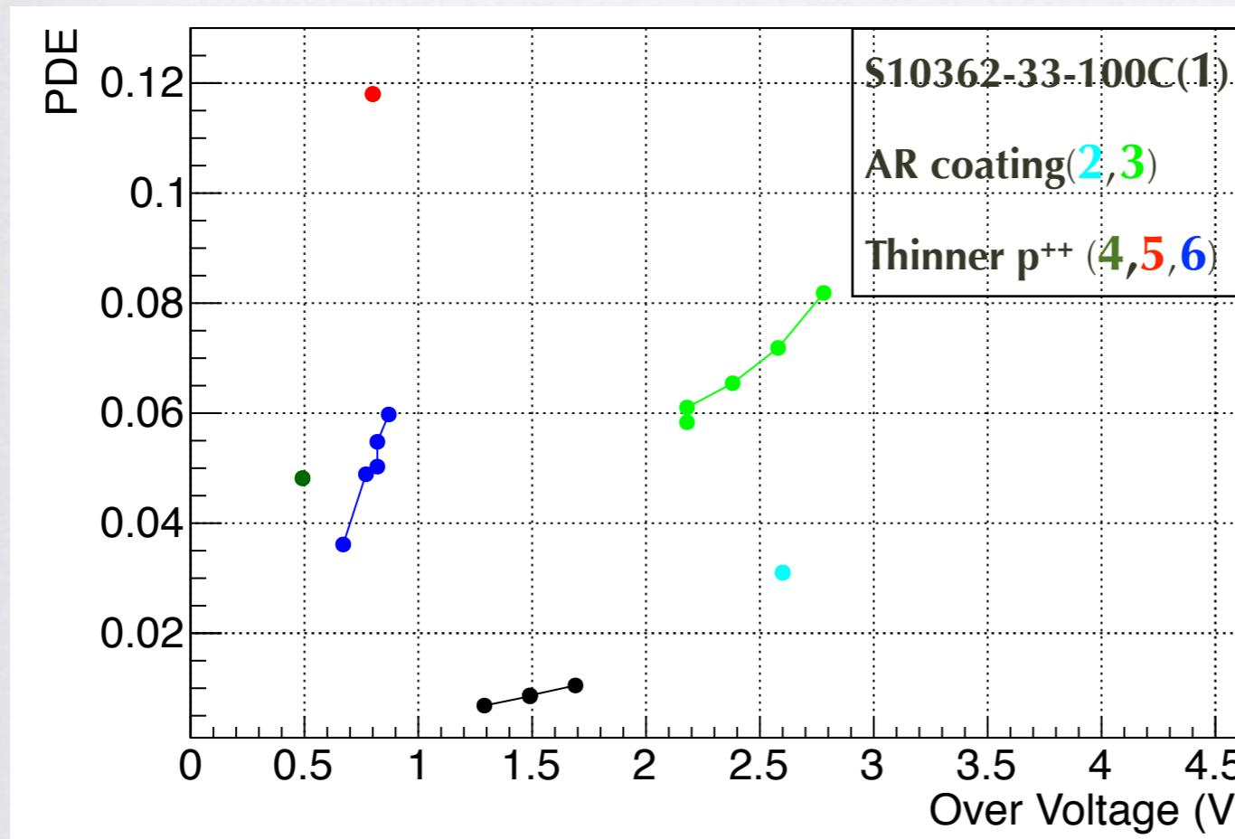
We confirmed PPD can be sensitive to VUV by removing protection layer and by making thinner p<sup>++</sup> layer.
