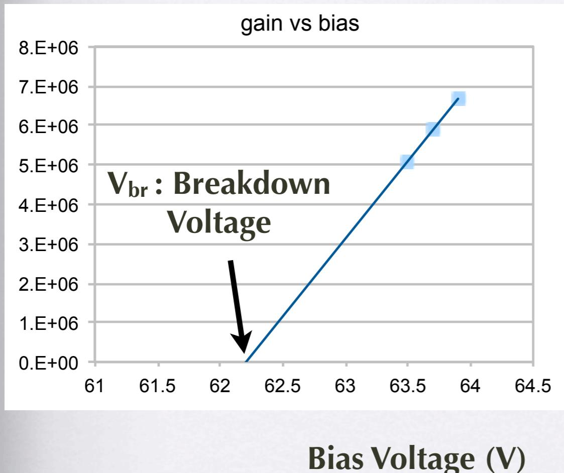
$$\text{Gain} = C(V_{op} - V_{br})/e$$
