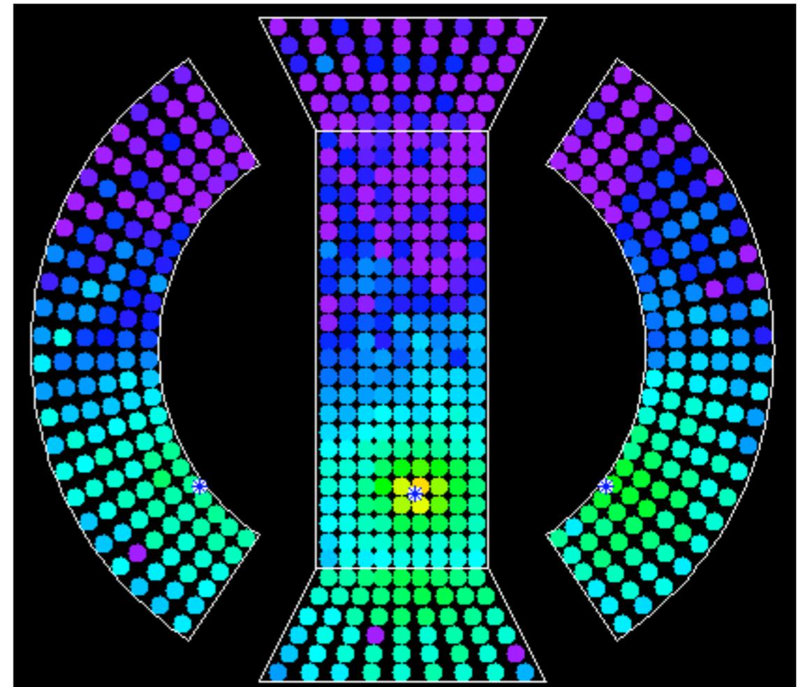
Energy of pileup gamma is estimated from information of main gamma. Only a part of PMTs are replaced, and most of original information is used for reconstruction
