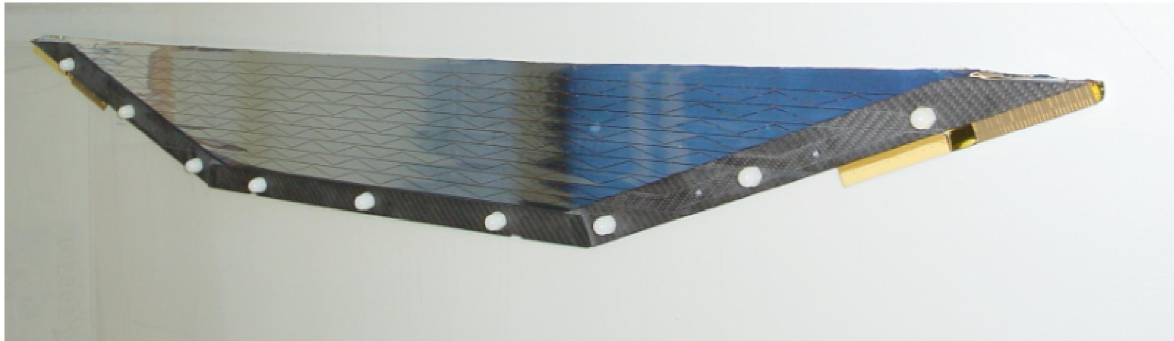
Inner cathode foil is mounted on the frame
