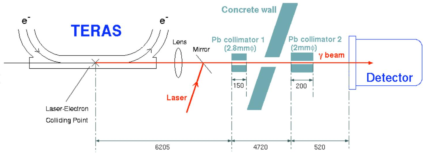
Photon beam is collimated by 2 collimators, and incident center of detector window.
