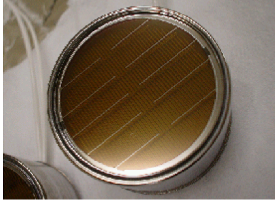
Figure 44: New PMT with an aluminum grid under the photocathode.
